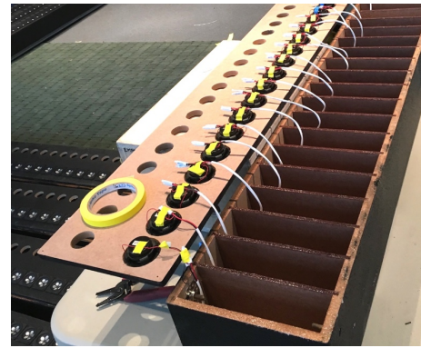
Figure 5 – Speaker installation, with openings for port tubes and internal subdivisions.
