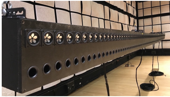
Figure 1 – Linear configuration with 5.8 cm distance between drivers.
